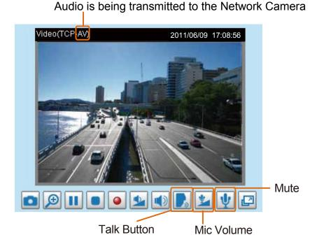
Click to enable audio transmission to the Network Camera; click to adjust the volume of microphone; click to turn off the audio. To stop talking, click again.
